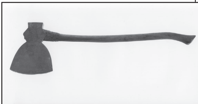
Figure 18e—A 19th-century shipwright's mast broad ax.
