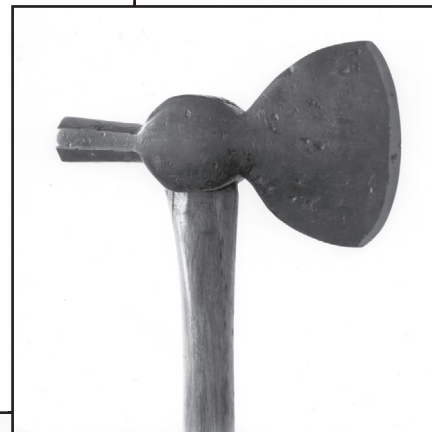
Figure 7—An 18th-century shingling hatchet is another specialized ax. Ax head is 5\frac{1}{2} inches long by 4 inches wide.
