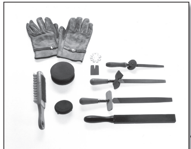
Figure 63 —Tools for sharpening (clockwise from top left) include leather gloves; ax-bit width gauges; 8-inch, 10-inch, and 12-inch mill bastard files; Carborundum scythe stone; Carborundum ax stone; file card; and grooved Carborundum sharpening stones. Natural Arkansas sharpening stones also work.
