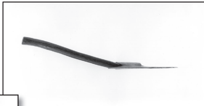
Figure 34b—A 19th-century S-bend broad ax handle.
