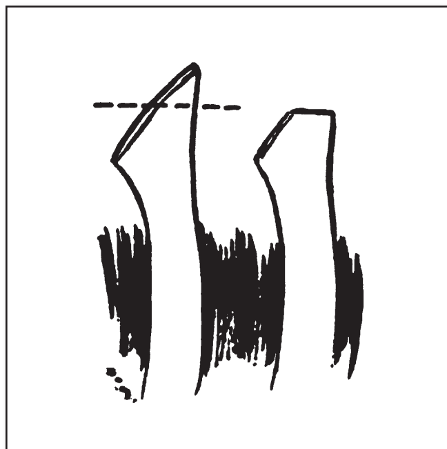
Figure 45—If you use a fawn's foot handle, saw off the handle about three-fourths of an inch from the butt end to provide a blunt surface for pounding with your mallet (drawing by Frederic H. Kock).
