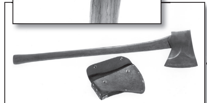
Figure 13—My favorite American felling ax, a True Temper Kelly Perfect with a Jersey head and 32-inch straight hickory handle. The scabbard is also shown.
