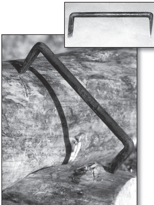
Figure 97—Use a log dog to secure the log to the yoke.
